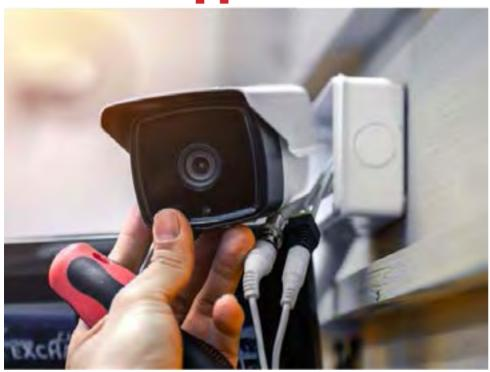
Wireless security camare closed-circuit television (CCTV) cameras that transmit a video and audio signal to a wireless receiver through a radio band. Many wireless security cameras require at least one cable or wire for power; "wireless" refers to the transmission of video/audio. However, some wireless security cameras are battery-powered, making the cameras truly wireless from top to bottom.
