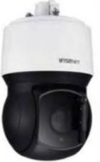
The new cameras uti-Hanwha Techwin, a lise an AI deep-learning algorithm for powerful object tracking (person or vehicle). Operators can simply right-click on an object to engage the target-lock tracking feature. The PTZ mechanism achieves a pre-set accuracy of ±0.1°, allowing the camera to move to the correct position within one second. The new dome design also enables significantly enhanced tilt angles, including 20° above the horizon and 90° straight down.
