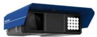
Hikvision, an IoT solution provider with video as its core competency, announced its latest traffic product offering - the All-Rounder ITS camera - designed to improve road safety and optimise traffic flow. As the name implies, the camera encompasses different skills and abilities, boasting speed detection, traffic violation detection, automated plate recognition, and vehicle attribute analysis in one housing.
